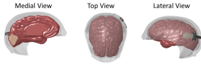
A 60-channel subdural electrode array creates phosphenes by stimulating neurons in the primary visual cortex.
