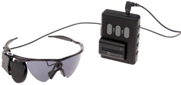
Figure 4: External Components of the Argus II System
