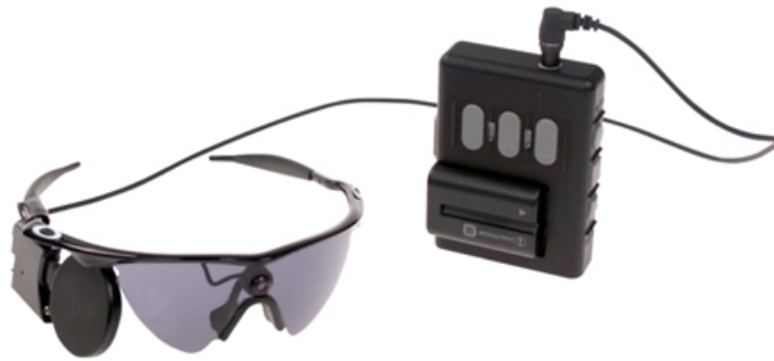
Figure 4: External Components of the Argus II System
