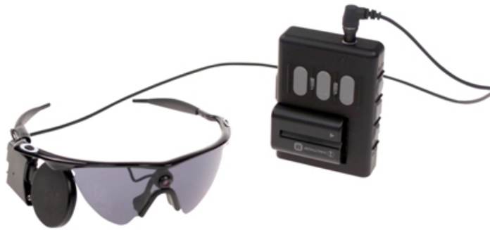
Figure 4: External Components of the Argus II System
