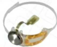
Argus II Implant – Electronics & 60 Electrode Array
